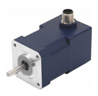
High-torque stepper motor with M12 connector with protection class IP65 (except shaft output) in size NEMA 17 (42 mm) and 1.8° step angle (full step). Identical flange size as the standard motor ST4118, therefore electrically and mechanically interchangeable.
