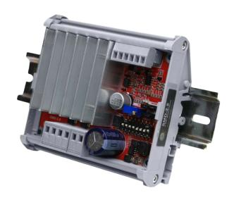
Stepper motor driver SMD-2.8 with DIN clamp is manufactured in an open case. A frameless version of the driver is also supplied.
