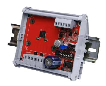
Stepper motor driver SMD-1.6 with DIN clamp is manufactured in an open case. A frameless version of the driver is also supplied.
