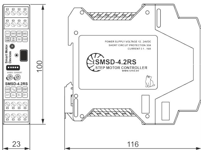
SMSD-4.2RS is a programmable step motor controller with RS-232 and RS-485 communication interfaces.
