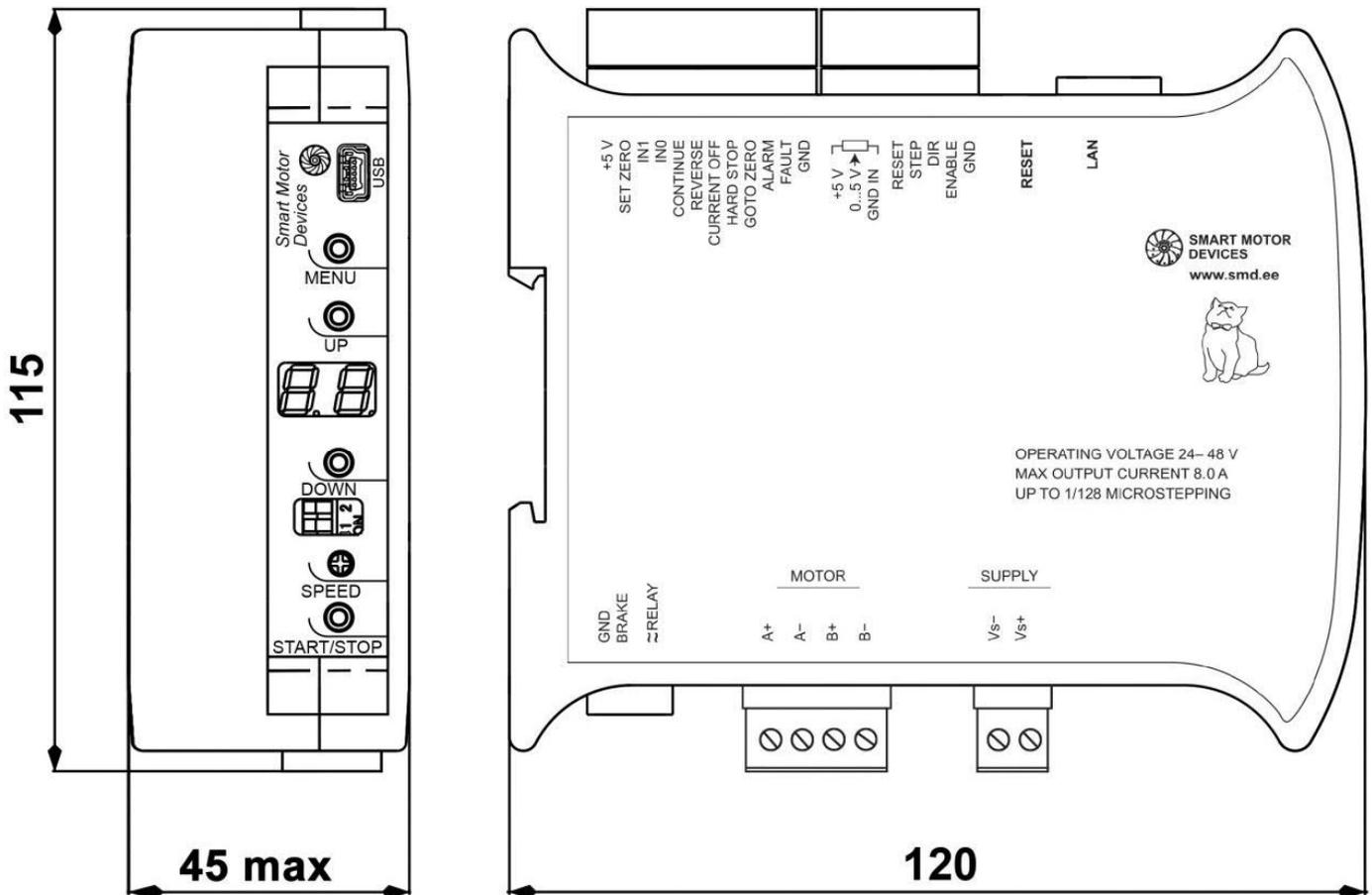
Fig. 1. Dimensions and input/output and controls location – SMSD\_LAN
