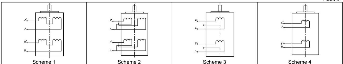
8 wires steppmotor connection (4 phases):
