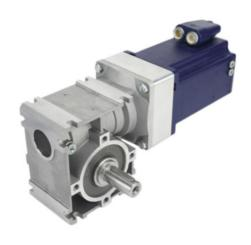
The GSGE80 gearboxes are intended for motor NEMA 34 (86 mm flange size). The output shaft is located 90° from the motor shaft. Worm gearboxes are characterized by self-locking and characterized by high efficiency. GSGE gearboxes come with a long-term synthetic lubricant, and are therefore maintenance free. The gearbox can only be ordered with a motor.
