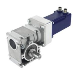
The GSGE60 gearboxes are intended for motor NEMA 23 (57 mm flange size). The output shaft is located 90° from the motor shaft. Worm gearboxes are characterized by self-locking and characterized by high efficiency. GSGE gearboxes come with a long-term synthetic lubricant, and are therefore maintenance free. The gearbox can only be ordered with a motor.
