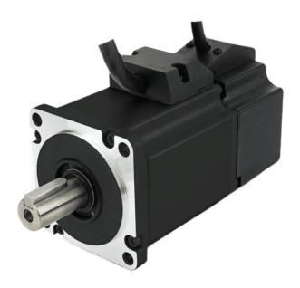
With rated power of 200 W, the high-performance BLDC motor APBA60M048030-E not only matches the power of AC servo motors with 60 mm flange but are also mechanically compatible. The DC motors are rated IP65 and comes standard with integrated encoder. The incremental encoder resolution is 2,500 CPR (10,000 PPR).
