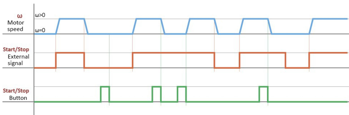
Fig. 5. Diagram of the coordinated operation of the external signal "START/STOP" and the built-in button.
