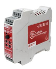
BLDC driver BLD-20DIN is a device designed to control 3-phase DC motors with Hall sensors. BLD-20DIN controls motor speed, acceleration and deceleration, direction. The controller has current limiting function to protect a motor.
