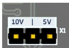
Fig. 7. 10V / 5V jumper.
