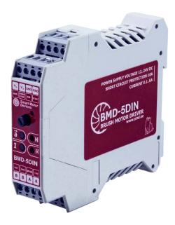
BMD-5DIN is a driver designed to control speed, direction, acceleration and deceleration of DC brush motors.
