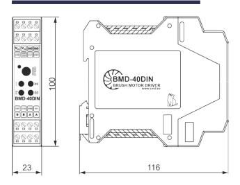
BMD-40DIN is a driver designed to control speed, direction, acceleration and deceleration of DC brush motors.
