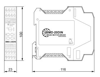
BMD-20DIN is a speed driver for DC brush motor. Motor speed is regulated by 0...5 VDC analog signal or can be adjusted by an internal potentiometer. Acceleration and deceleration time are also adjusted by potentiometers. The controller provides current limitation function to prevent motor overloading.
