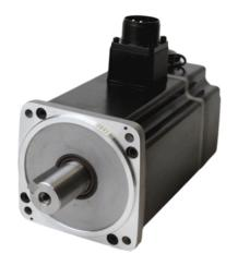
The output power of 5000 W fits into a servo motor EM3A-50 with a flange size 130 mm. This motor has low rotor inertia and high speed, suitable for highly dynamic systems. Movement accuracy is ensured by modern optical or magnetic encoders with a resolution of up to 23-bit. Products can be provided with a 24VDC holding brake option.
