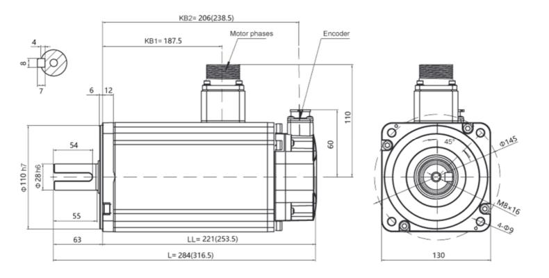
Note: The values in parentheses represent the values of motors with brakes
