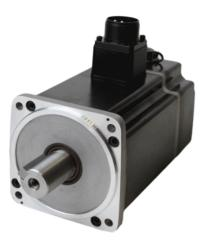
The output power of 4000 W fits into a servo motor EM3A-40 with a flange size 130 mm. This motor has low rotor inertia and high speed, suitable for highly dynamic systems. Movement accuracy is ensured by modern optical or magnetic encoders with a resolution of up to 23-bit. Products can be provided with a 24VDC holding brake option.
