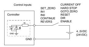
Fig. 3. Connection of input lines using external power supply (4-5VDC).
